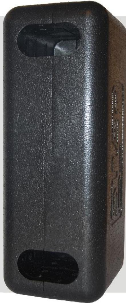
This insulation for heating applications consists of 2 half-shells and is made of expanded polypropylene. Due to the half-shell system, the assembly on the already installed heat exchanger is possible.
