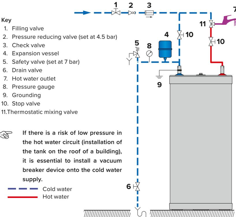
**CONNECTION TO THE PRIMARY CIRCUIT (Typical floor installation)**
